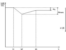
These measured quantities are required for type testing for electrical operating equipment per IEC/EN 61000-3-3. Adherence the limit values set forth in this standard is required as of the year 2001 for application of the CE mark to electrical and electronic equipment and devices with input current of up to 16 A.
