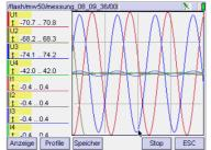
In addition to acquiring sporadic mains voltage interferences, this type of representation is especially well suited for recording current and voltage signal characteristics when power consumers are switched on and off (e.g. motor start-up).
